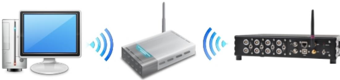
This mode is supported by the CAP and the 4X. Before operating the CAP/4X must connect to the same Wi-Fi network of the computer.
