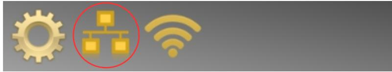
The Ethernet configuration dialog is activated if the second button on the bottom bar is pressed.
