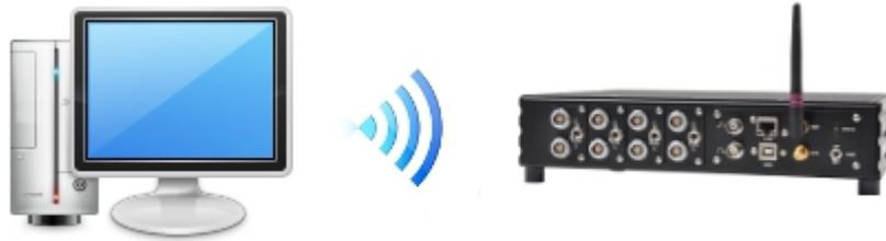
In this case the device behaves as an access point and the computer must connect to its Wi-Fi network.
