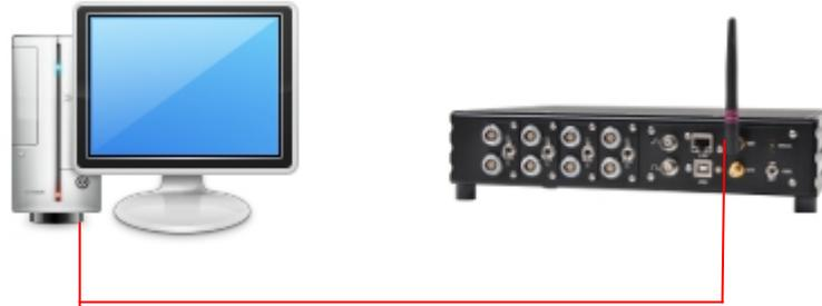
The direct connection to a computer requires the manual configuration of the computer and the device IP addresses. Both the addresses and sub-net masks must be compatible to each other.
